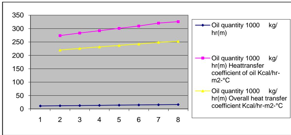
Fig.3 Variation of heat load and overall heat transfer coefficient with oil quantity
