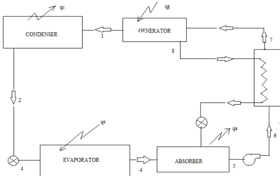
Fig.1 The schematic of the absorption refrigeration cycle.
