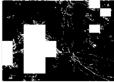
Final output after filtering showing the weed affected areas as white blocks.
