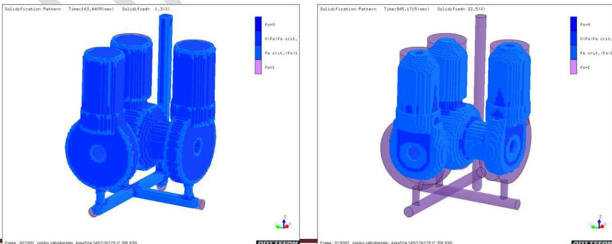
The results obtained from iteration 2 shows that there is no shrinkage occurring in the valve body. Thus it can be concluded that the results obtained from iteration 2 i.e. bottom gate with the aid of chills produces defect free casting. Thus there is no need of next iteration.
